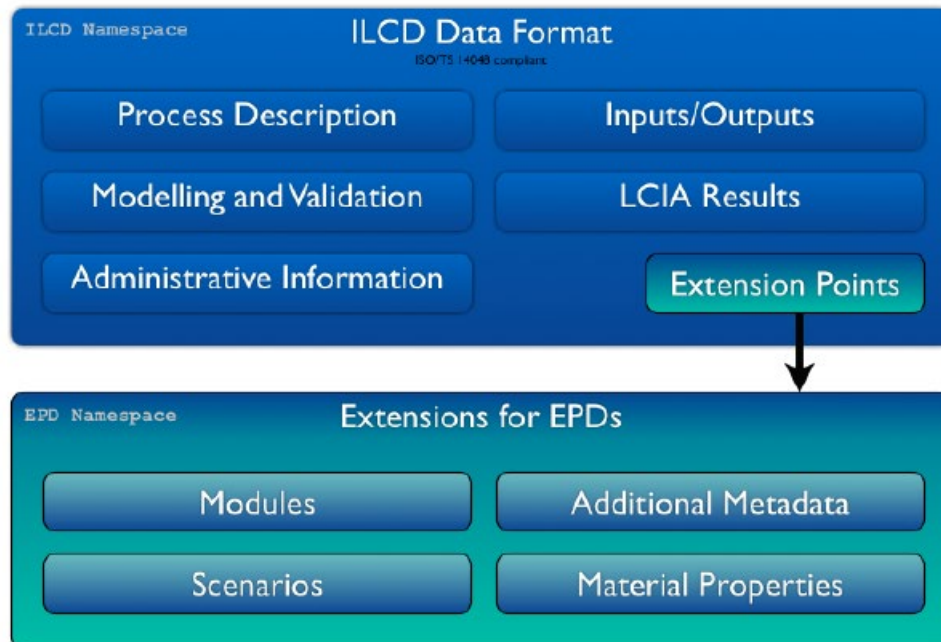
Figure 3. Conceptual presentation of the ILCD+EPD data format (Ökobau.dat, 2017).
