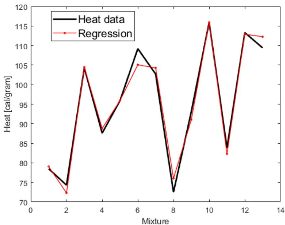
Figure 2 Heat data for cement mixtures containing four basic ingredients.
